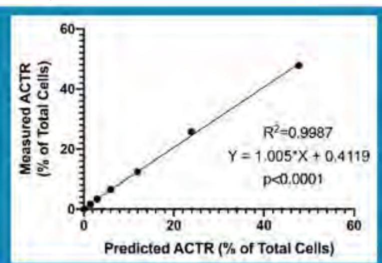
Linear dilution series analyzed on the Accellix platform. A linear regression analysis showing excellent dilutional linearity when the measured frequency of ACTR+ cells is compared against the expected concentration of each dilution. An R2 value of 0.9987 was observed.
